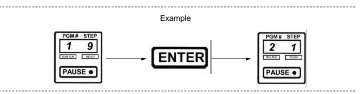
To edit a recipe or to correct mistakes, use the same step above to enter the programming mode, then push "ENTER" to reach the program/step that you wish to edit.
